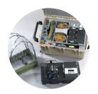
A leakage isolation test allows the operator to isolate the location of a leak and possibly remedy the situation; thereby permitting the continued fielding of the mask. Mask components that are prone to leaks include: voicemitters, exhalation ports and disks, inlet port seals, and drink hoses and couplings.
